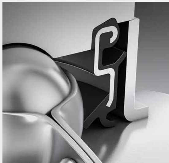
An inner ring installed slinger and advanced double-lip contact seal form a virtually impenetrable barrier to contaminants
